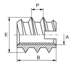
Female thread A = M16Length B = 26Male thread E = 24.0Min hole depth = 30
